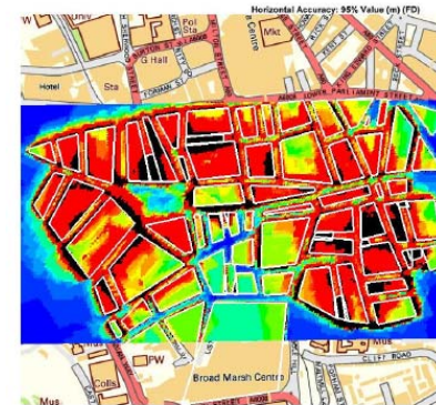
Figure 21 High Sensitivity GPS performance
