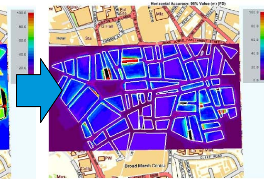
Figure 22 High Sensitivity GPS + Galileo performance
